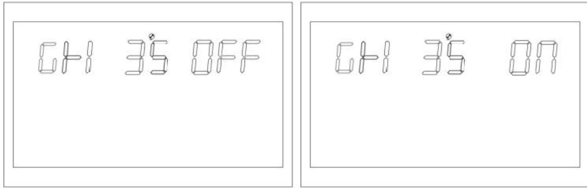
Figure 4.6-33 Grid-tie inverter function setting page
