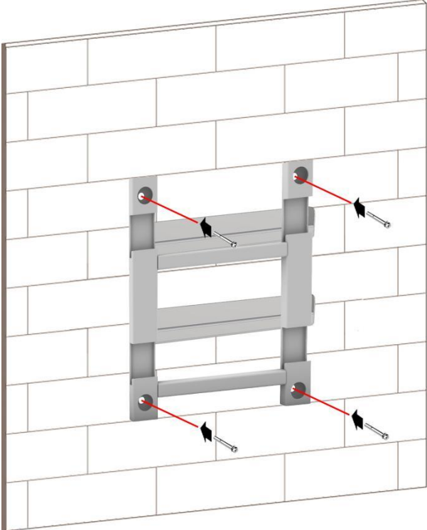
Figure 2.1-3 Install the wall bracket
