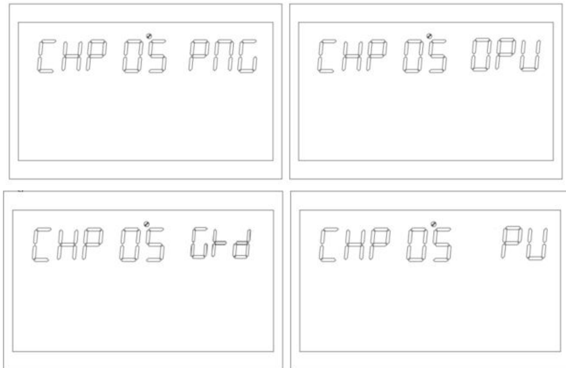
Figure 4.6-5 Charging priority setting screen
