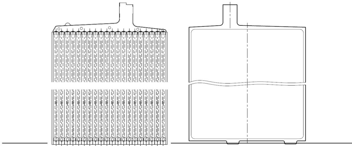
Positive tubular plates and negative flat plates are standing on ground on the container. The negative plate has 10mm high feet casted with the grid and the positive plate has a plastic bottom bar, with a height of 6mm inside and 6mm outside of the tubes.
