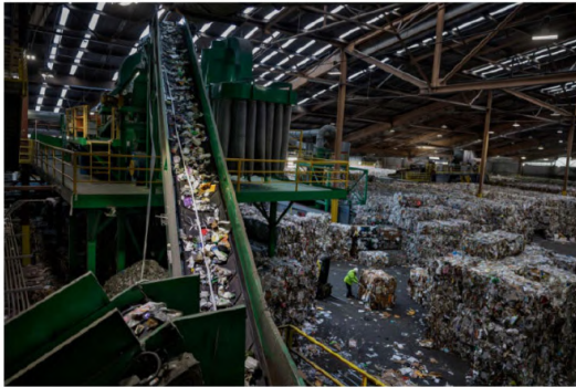
A conveyor belt carries mixed plastic to an optical sorter. PHOTOGRAPH BY RANDY OLSON, NAT GEO IMAGE COLLECTION
